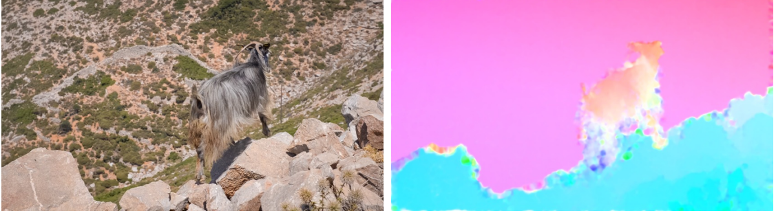
Figure 2.3: Optical Flow computed using Farneback's algorithm [22] and visualised using the colour encoding presented in [2].
