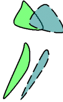
FIGURE 2.14: Possible effect of insufficient sampling. Overlap-based algorithms will fail to track the bottom feature [19]
