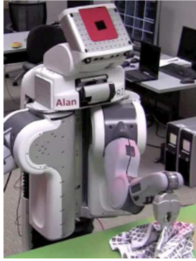
(a) Robot grasping garment from a pile
