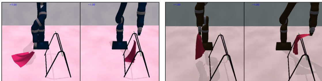
Figure 7.1: Cloth anchored to the gripper to create fake grasp before our code changes (left) and after (right)
