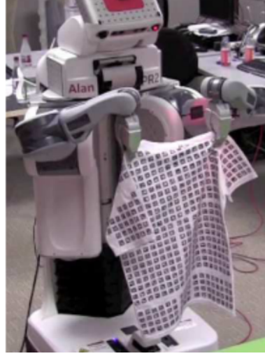
(b) Robot holding the garment with fiducial marks visible
