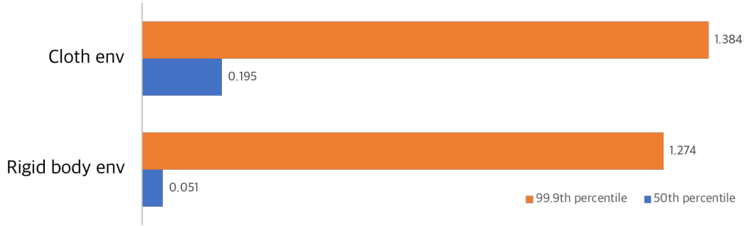
Figure 7.3: Comparison of wall time of execution (in seconds) of one simulation step between Hanger environment (cloth env) and Reacher environment (rigid body env).
