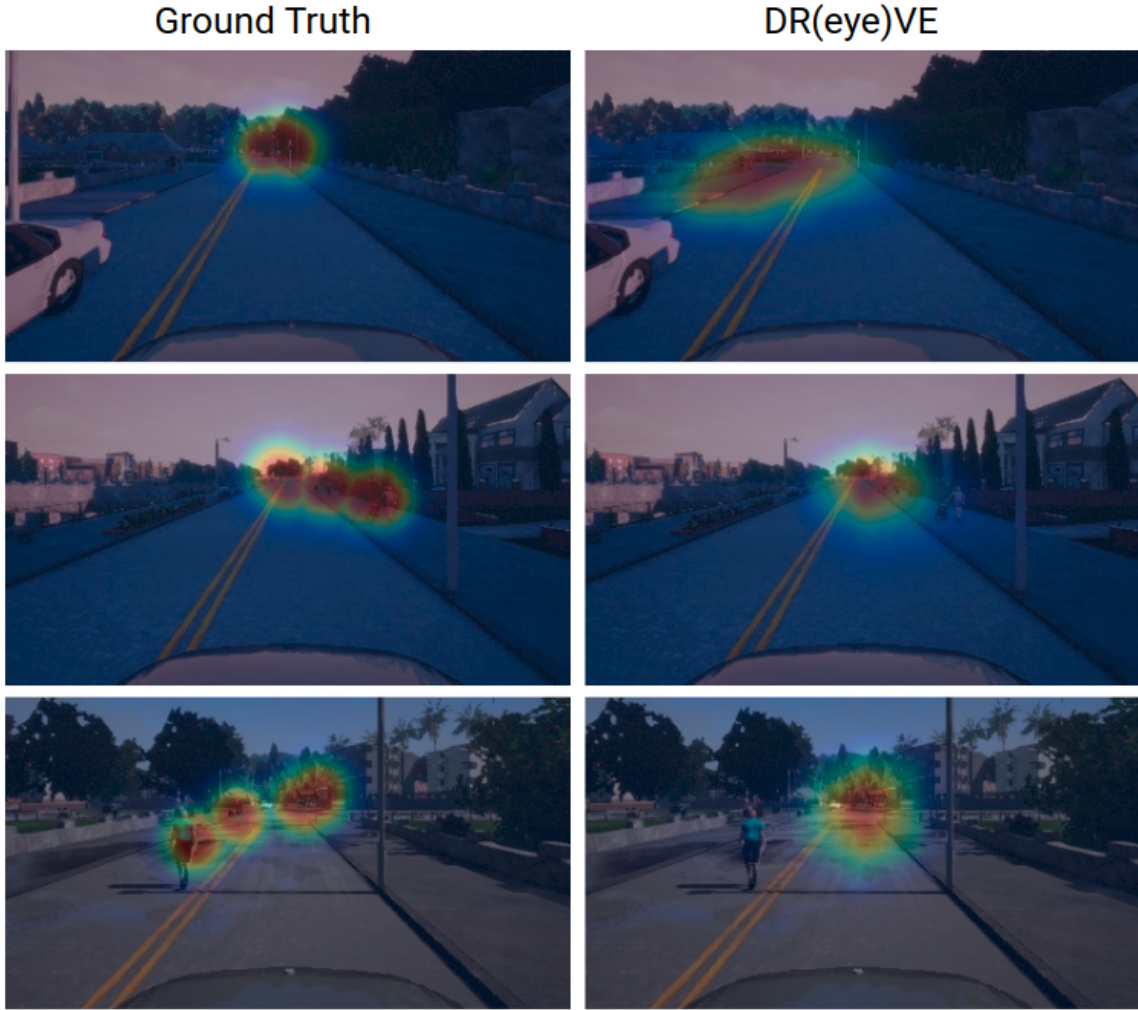
Figure 5.12: Some failure cases for the DR(eye)VE model. In the top image, the model is looking behind the oncoming car rather than at the road ahead of it, while in the center and bottom images it ignores pedestrians which the human driver chose to look at.
