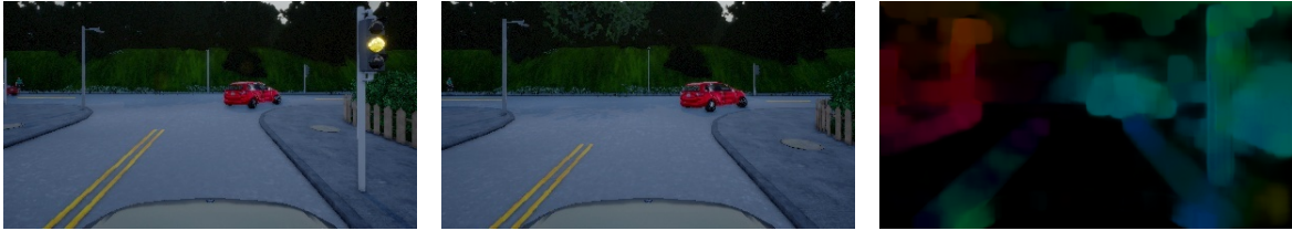
Figure 3.5: Farneback dense optical flow map produced by two camera frames separated by 3 time steps
