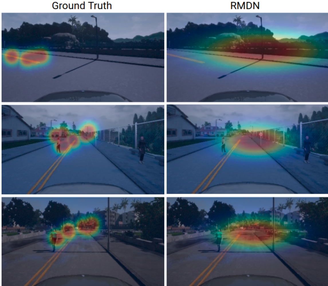
Figure 5.5: Sample test set predictions from the fully trained RMDN Model. Clearly having overfit to the mean of the dataset, RMDN gives very inflexible and uninformative predictions, missing key features such as the pedestrians in the middle and bottom images.
