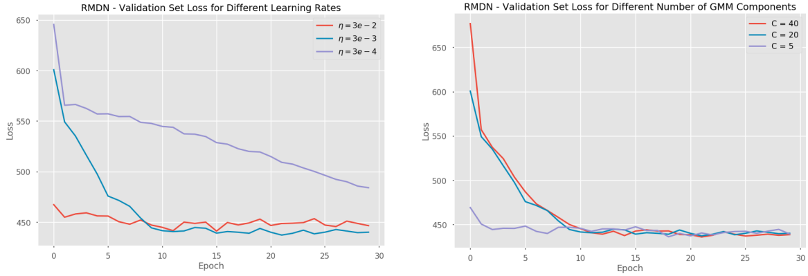
Figure 5.4: Comparison of validation loss for (left) 3 different learning rates and (right) 3 different numbers of GMM components for the Recurrent Mixture Density Network
