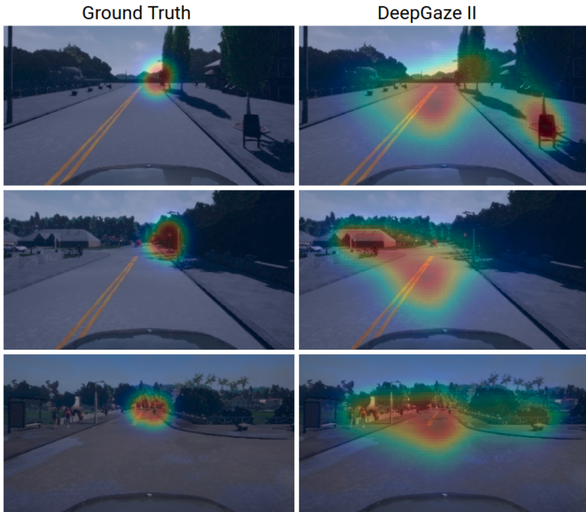
Figure 5.1: Sample test set predictions from the pre-trained Deep Gaze II Model. Note how the model predicts fixations for unimportant objects such as the mailbox in the top figure and the house in the middle figure, showing its lack of task-specific knowledge.
