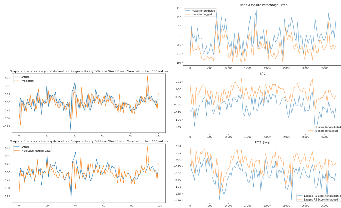
Figure 10.3: Visual inspection of lag(left) and Metrics plotted against time(right) for the Hourly Belgium Offshore Power Generation Dataset.
