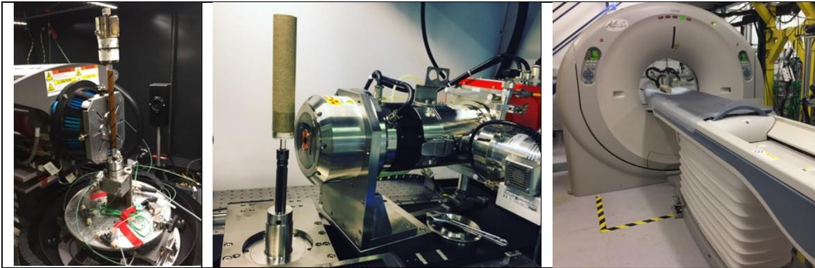
Figure 2. The multi scale X-ray imaging and experimental core flooding facility at Imperial College London with micro X-ray CT (left, centre) and medical X-ray CT (right)
