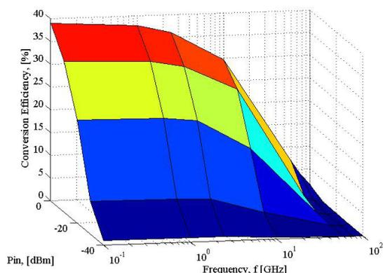
Figure 3 MZBD-9161 impedance matched series configuration results.
