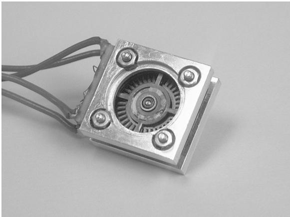
**Figure 5** MEMS axial flow turbine generator (approximate size 15 x 15 mm).
