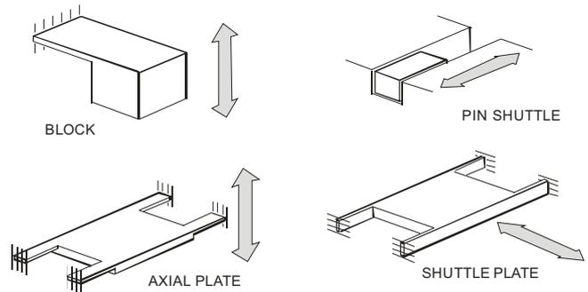
**Figure 2:** Principal proof mass and suspension geometries for inertial energy harvesters.
