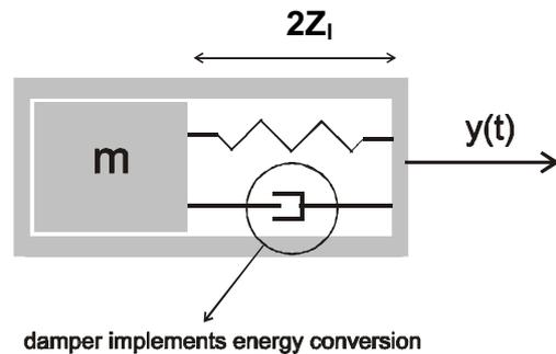
**Figure 1:** Schematic of linear inertial energy scavenger. A spring suspension supports a proof mass  $m$  within a frame, motion of the mass on its spring is excited by motion of the host structure  $y(t)$ , and damping of this internal motion by the transducer generates electrical power.
