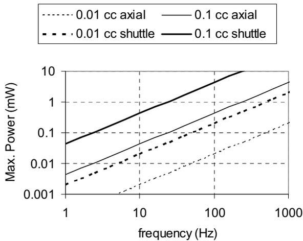
**Figure 3:** Maximum power levels for MEMS inertial energy harvesters of axial plate or shuttle plate geometries, for proof mass volumes as indicated.
