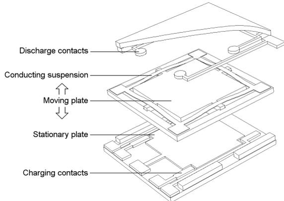
**Figure 4** MEMS Electrostatic energy scavenger for low frequency applications (from [7]), using a Si proof mass on a polyimide suspension.
