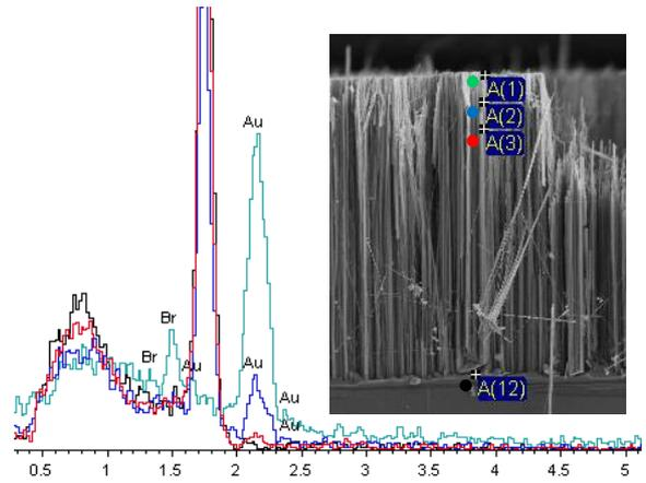
Fig. 5 Energy dispersive X-ray analysis along the cross section of the NW array. The X-ray was spotted at the dotted area shown in the inset. The Au can only be found on the top 10  $\mu\text{m}$  of the NWs.
