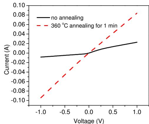
Fig. 3 Current-voltage characteristic of a p-type NW array with Cr/Au as top and bottom contacts. Contacts become Ohmic after anneal at 360 °C for 1 min.
