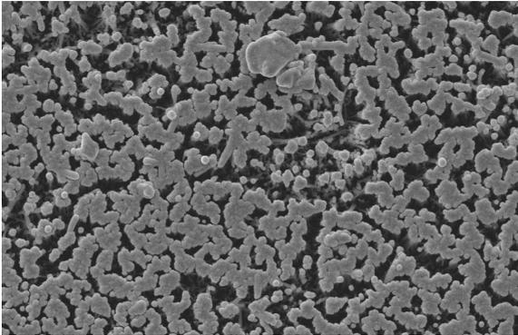
Fig.4 SEM picture of the top of the metallised Si NW array
