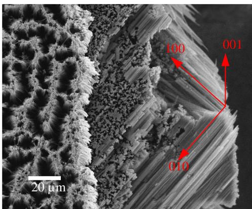
Fig. 2, SEM image of the NW arrays etched at the cleaved edge of the wafer.
